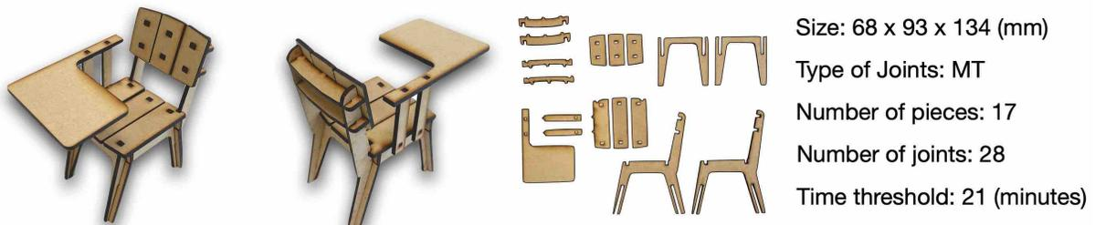
Figure 16: Details of each chair used as our representative laser-cut architecture examples. In a top-down order, the chairs were named based on the types of joint: Finger, Slot, MT, FingerMT and SlotMT in this paper.
