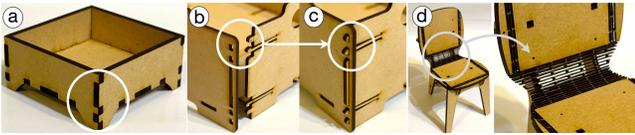
**Figure 10: Implementations of potentially accessible joint designs. (a) Fingers with distinct widths (Modified from thing:2250238). (b) SpringFit [71] joints allow more manipulation room to snap-fit the joint (c) and generate a haptic click once connected (thing:333047). (d) Living hinges can bend to form a corner without effortful assembly (Link to model).**
