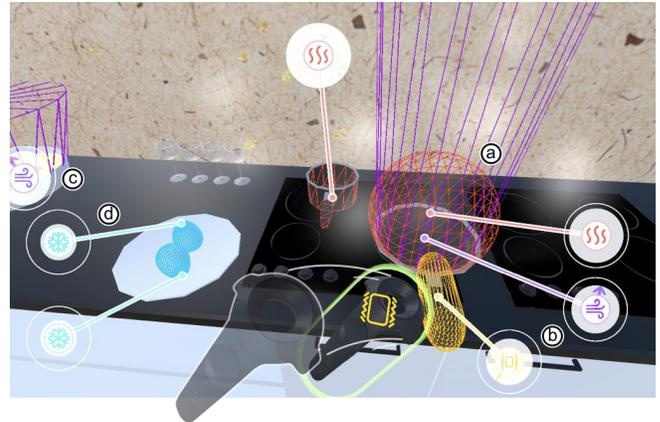
Figure 1. The visualization design of SeeingHaptics. (a) Wireframe of haptic area. (b) Haptic type and properties shown on an icon. (c) Repositioning outside icon. (d) Radially shift inside icon to peripheral vision.
