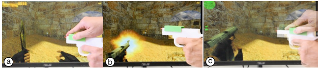
Figure 9. (a) In the FPS game, a user browses the available weapons using the slider on the top of a toy pistol, (b) shoots by pressing the trigger, and (c) reloads the bullets by pushing or pulling the slider.
