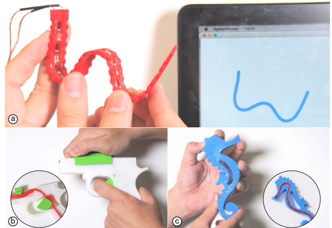
Figure 1. (a) FlexiBend is an easily installable shape-sensing strip that enables interactivity of (b) multi-part, (c) deformable fabrications.
