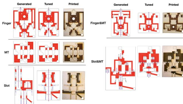
**Figure 9: *Daedalus*-generated SVGs (left), tuned SVGs by an occupational designer (center) and printed laser-cut plates with assembly components removed (right). Dotted lines indicate layer-local and within-component lines of symmetry in the *Daedalus*-generated layouts, and global lines of symmetry in the tuned layouts. (Note: the MT layout and the top of the SlotMT layout do not have lines of symmetry, because these model parts are inherently asymmetrical.)**
