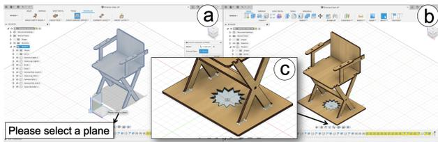
Figure 6: Workflow for adding support area. (a) *Daedalus* asks the user to specify the plane for locating the support to be placed. (b,c) *Daedalus* captures the footprint of the chair automatically, and adds the ground support area with a hollowed star to the authoring space.
