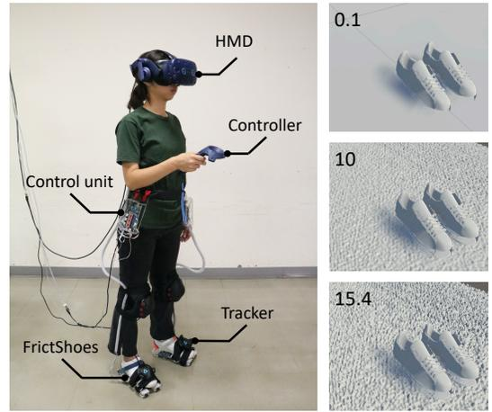
Fig. 7. The setup of magnitude estimation study (left) and ground roughness for minimum, moderate and maximum scale (right).
