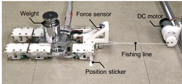
Fig. 6. The setup for measuring maximum static friction force.
