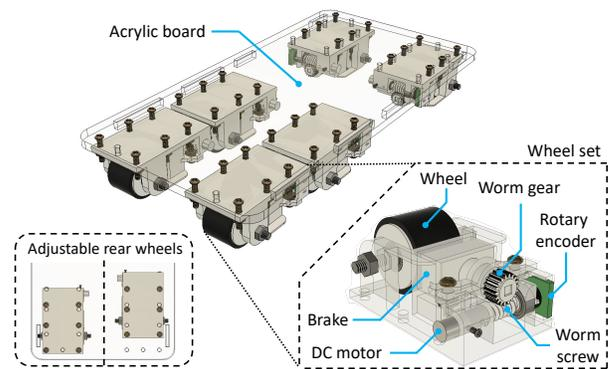
Fig. 3. The 3D model of the current FrictShoes prototype.
