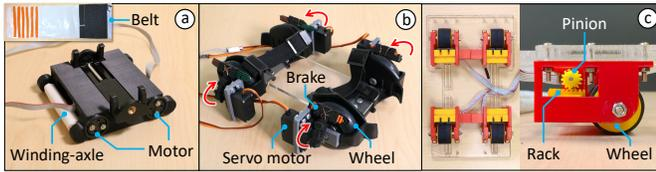
Fig. 2. The preliminary prototypes used the (a) material-switching concept, (b) braking control mechanism, and (c) rack and pinion mechanism.
