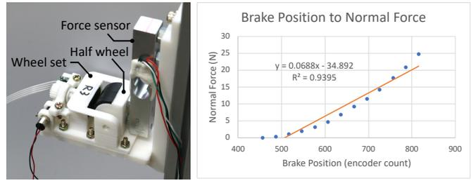
Fig. 5. The setup for measuring normal force (left) and the relationship between the brake position and normal force (right). The sampled force at different positions and the linear regression line are shown.
