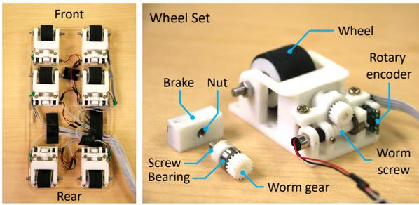
Fig. 4. The FrictShoes device. The bottom view of a FrictShoe (left) and the wheel set with an exploded view of its parts (right).
