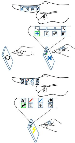
**Figure 1:** In SegTouch, buttons are assigned to different positions on the index finger to provide mode switching. Top: in 3D navigation, users swipe in conventional touch to rotate and swipe with SegTouch to translate. Down: tool buttons in reader and text editor.
