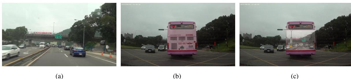
**Figure 1:** A synthesis result of the proposed view sharing system. (a) The original view of the preceding vehicle. (b) The original view of the subject vehicle with a large portion of the image blocked by the preceding vehicle. (c) The perspective of the preceding vehicle is transferred to the corresponding view of the subject vehicle to “disocclude” the blocked area as if the preceding vehicle becomes transparent.
