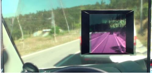
**Figure 2:** Previously proposed See-Through System (STS) presents to the driver a view with images taken from the preceding vehicle directly super-imposing over the image area occupied by the preceding vehicle [GVF12]. However, the drivers need to pay extra attention since the perceived contextual information from different views are highly inconsistent.
