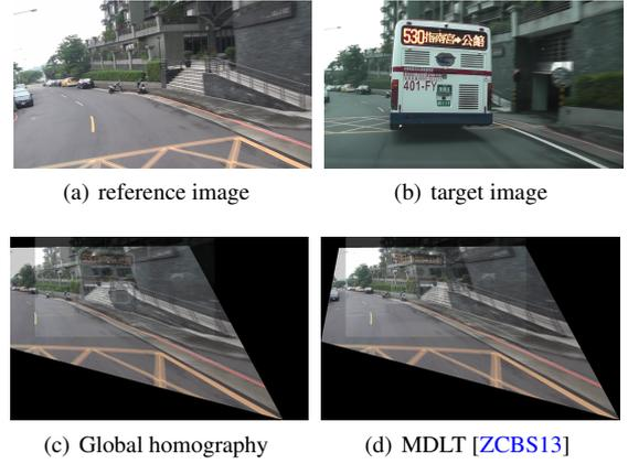
**Figure 5: Aligned images.** (a) reference image captured by the preceding vehicle. (b) target image captured by the subject vehicle. (a) and (b) are input pairs. (c) the synthesized result stitched with global homography after final stitching. (d) the synthesized result stitched with MDLT method after final stitching.
